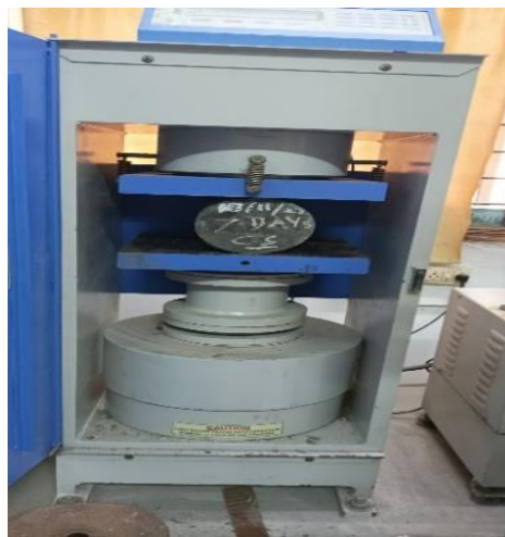
Fig 6.5 Split Tensile Test
