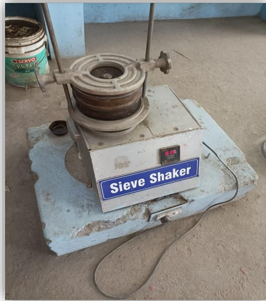
Fig. No.4.4: Sieve Shaker (Fineness Test) Fig. No.4.5: Fineness Test on Cement
