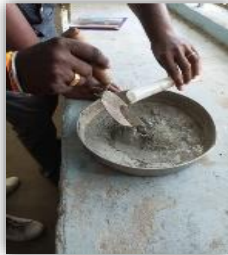
Fig. No.4.8: Setting Time of Cement
