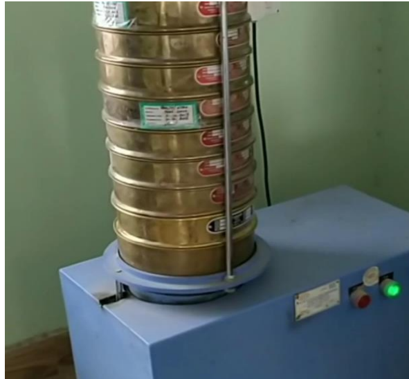
Fig.4.9. Sieve Analysis Test.
