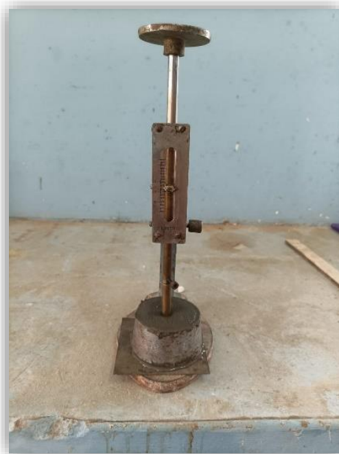
Fig. No. 4.6: Normal Consistency Test using Vicat Apparatus.
