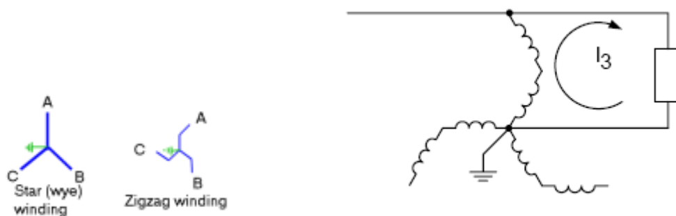
Figure 4.13. Zigzag transformer winding diagram
