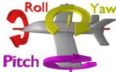
Fig 9 .Attitude degrees of freedom for an airplane.
