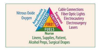
Before we undertake fire prevention, we first need to understand the three main ingredients that constitute a fire: heat, fuel, and oxygen. The paradigm below, referred to as the "fire triangle," shows how these three components interact to create a fire
